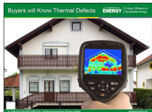
IR camera finds thermal leaks
